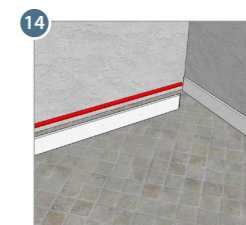
14 Bonding of decorative strips and skirtings on walls COSMO® PU-100.110 COSMO® HD-100.480 Please find further information on page 26.
